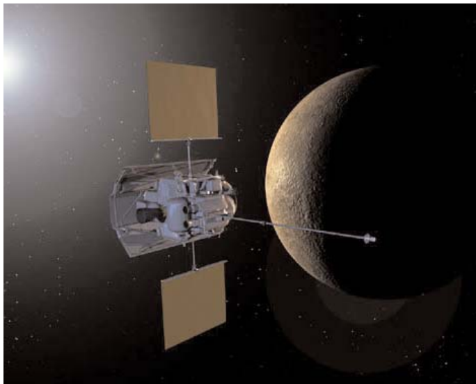
Figure 1. MESSENGER spacecraft with its solar panels angled toward the Sun for safe power generation.
